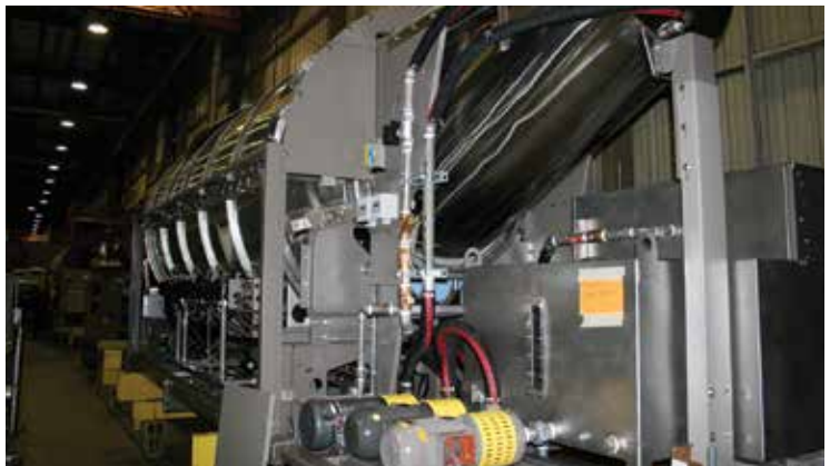
At left are tunnel washers under construction and a robotic laser for cutting metal at Pellerin Milnor's plant, located near Associated Hospital Services. Above (from left) are Milnor Vice President of Product Development Russell Poy, Plant Manager Henry Polk and Consultant Sam Garofalo.
