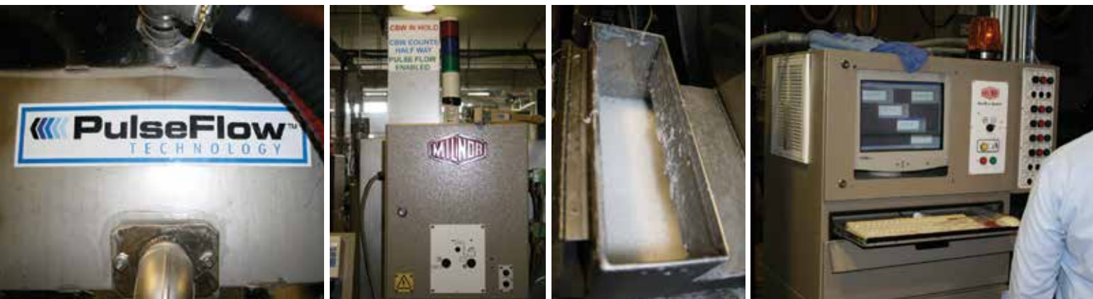
Above is Associated's new tunnel. The second image from left has an indicator light that shows when PulseFlow is deployed. Next to that is the inside of a level, or weir box, showing the suds level. At right is a Multitrac control system; it shows progress in other systems. Below is a view of the tunnel inverter.
